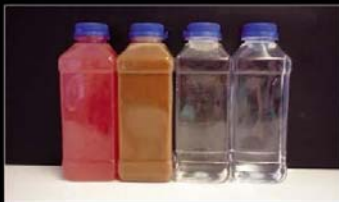
Samples showing untreated wastewater, biomass, AMBR treated water and post RO treated water.
